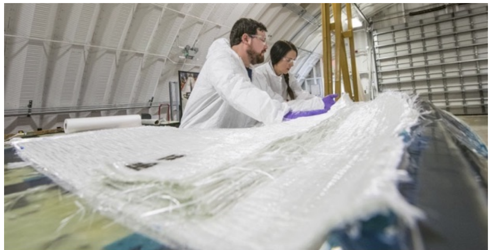
Figure 6 (left) and 7. Researchers at the National Renewable Energy Laboratory (NREL) construct a 13-m thermoplastic composite blade at NREL's Composites Manufacturing Education and Technology Facility. Photos by Ryan Beach, NREL
