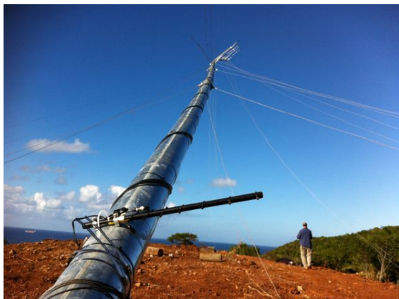
Anemometers are utilized to accurately measure wind speeds at proposed sites. Photo by Owen Roberts, NREL 23842.
