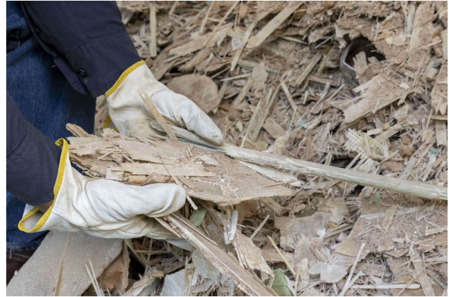
Figure 2 (left) and 3. The image on the left shows wind turbine blades being segmented for mechanical recycling at Veolia's blade recycling facility in Louisiana, Missouri. The image on the right is the final product that is realized when the mechanical recycling process is complete. Photos from Veolia
