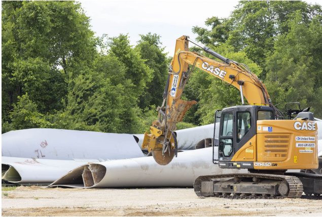
Figure 2 (left) and 3. The image on the left shows wind turbine blades being segmented for mechanical recycling at Veolia's blade recycling facility in Louisiana, Missouri. The image on the right is the final product that is realized when the mechanical recycling process is complete. Photos from Veolia
