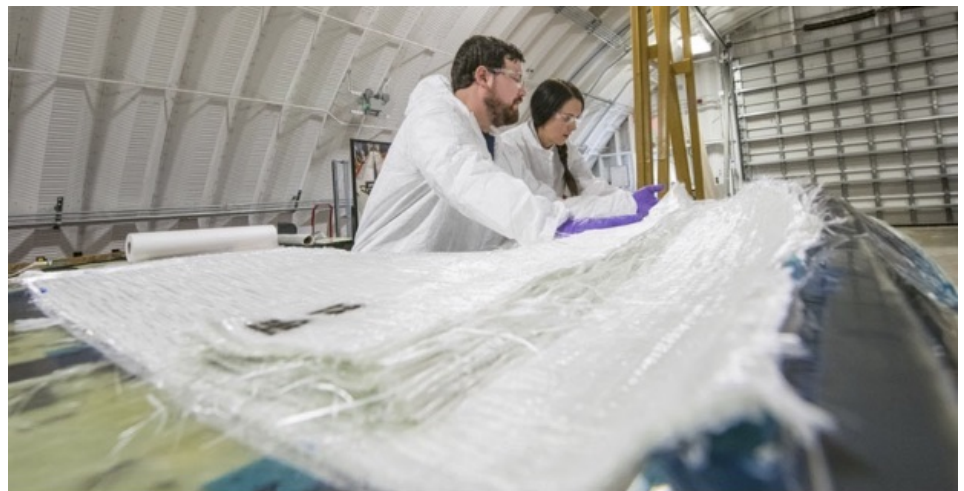
Figure 6 (left) and 7. Researchers at the National Renewable Energy Laboratory (NREL) construct a 13-m thermoplastic composite blade at NREL's Composites Manufacturing Education and Technology Facility. Photos by Ryan Beach, NREL
